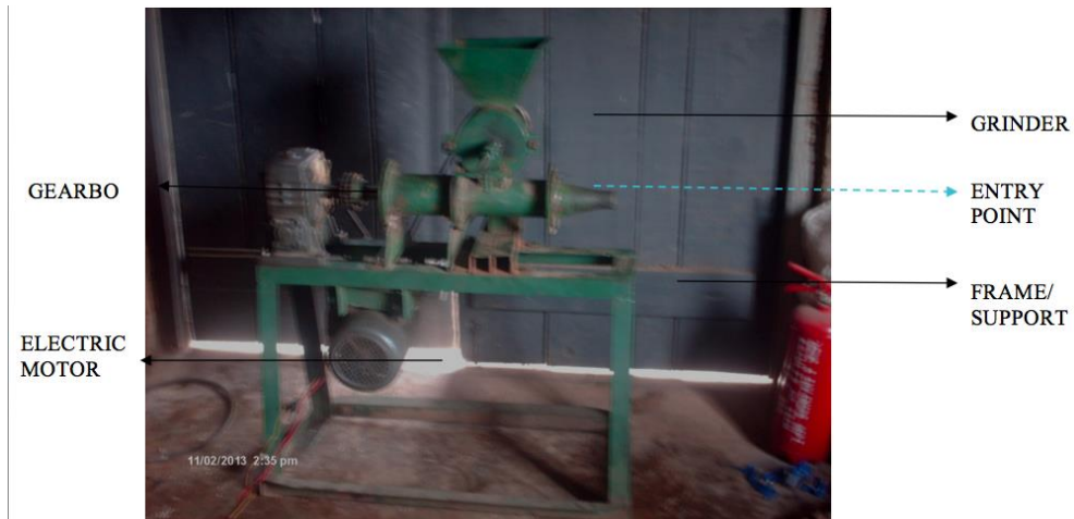
Plate 2: The Combined Grinding and Pelletizing Machine
